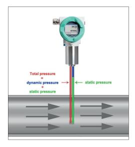
The integrated, precise differential pressure sensor measures the differential pressure/dynamic pressure at the sensor tip. The pressure depends on the respective gas velocity. The flow is therefore easy to determine by means of the pipe diameter.
