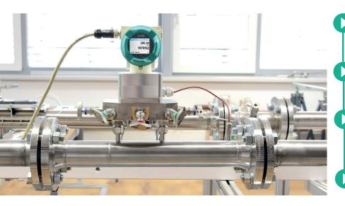
Reference measuring device for blower and compressor test benches (effective delivery capacity)
