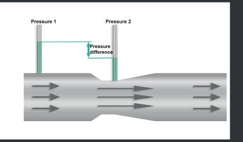
For differential pressure measurement, two separate lines lead to a differential pressure measuring cell. One pressure connection (pressure 1) is located at the inlet of the Venturi tube and a second pressure connection is located at the outlet of the Venturi tube (pressure 2). Without flow, the pressure at the inlet and outlet is identical.
