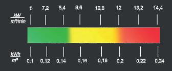
A typical specific power requirement of an oil-injected compressor can be as follows:
